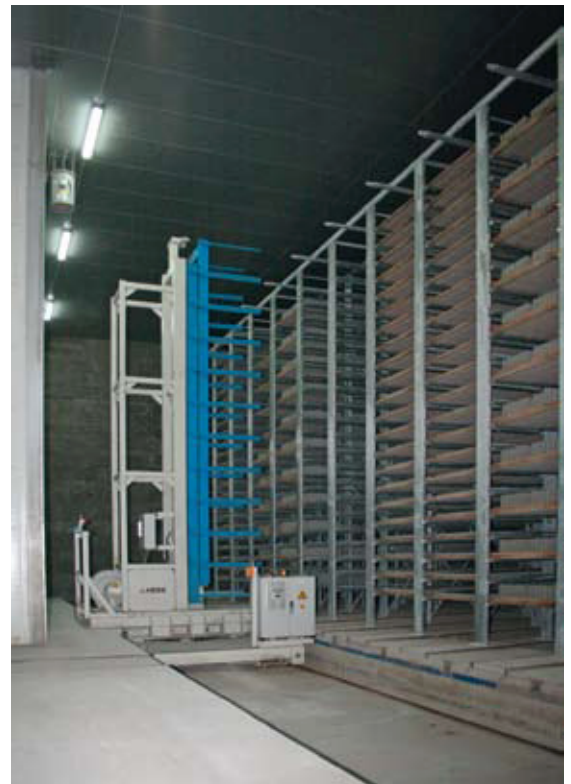
Fig. 5 Curing chambers supplied by Rotho provide space for 6,000 boards.
