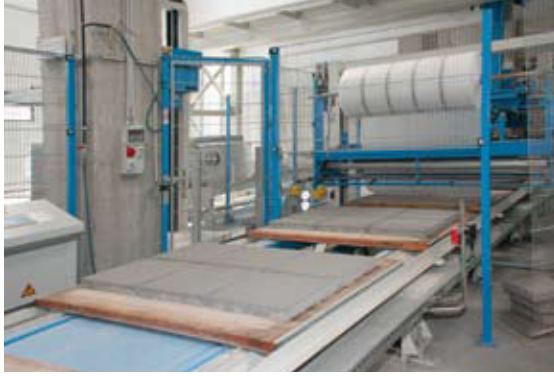
Fig. 7 Premium quality: A foam sheet is inserted on top of each layer.
